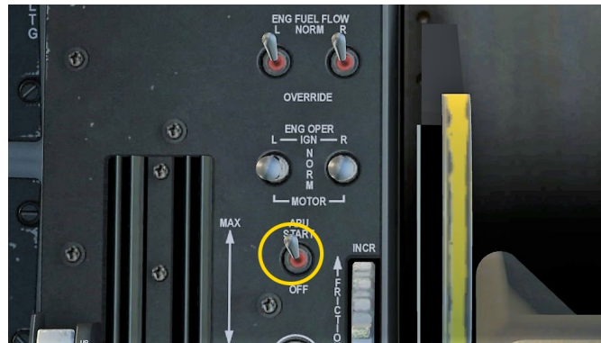
Figure 2.3: APU START under the throttle
