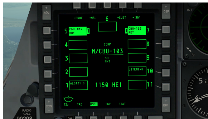
Figure 3.8: DSMS on left MFCD CBU selected
