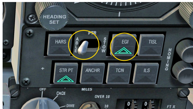
Figure 2.11: NAV Mode Select Panel on front dash
