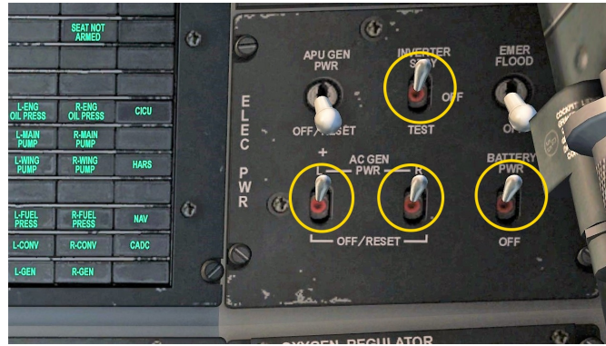
Figure 2.2: ELEC PWR Panel on the right side of the cockpit
