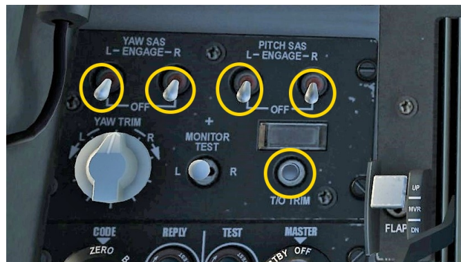
Figure 2.8: TRIM Panel on the left side of the cockpit
