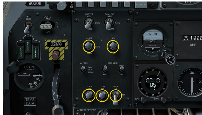
Figure 2.9: AHCP on the front dash
