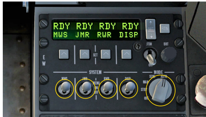
Figure 2.10: Countermeasure Panel on the right side of the cockpit
