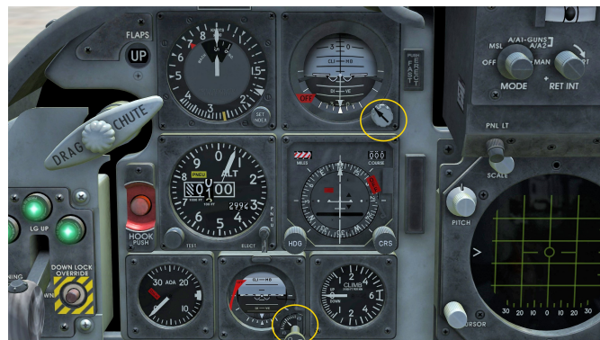
Figure 2.8: Front dash with attitude indicators
