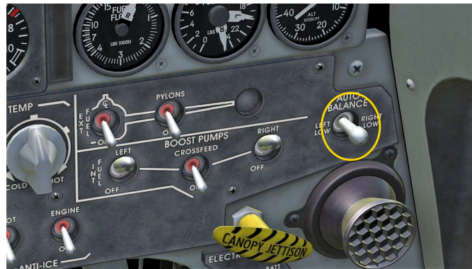
Figure 2.22: Balancing the fuel
