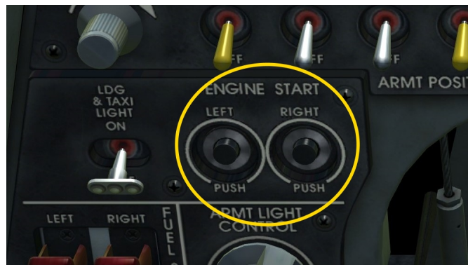
Figure 2.5: Engine starter buttons
