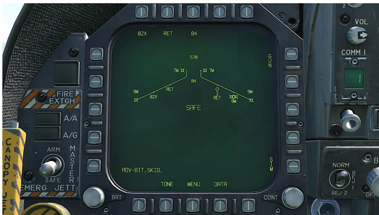
Figure 31. Stores Management System (SMS) Page
