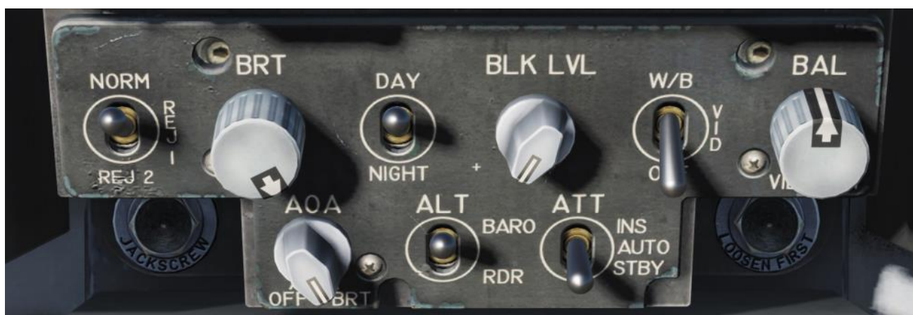
Figure 11. HUD Control Panel
