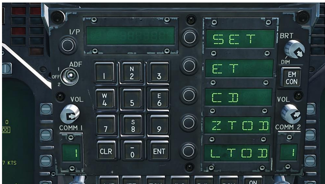
Figure 37. TIMEUFC Options on UFC
