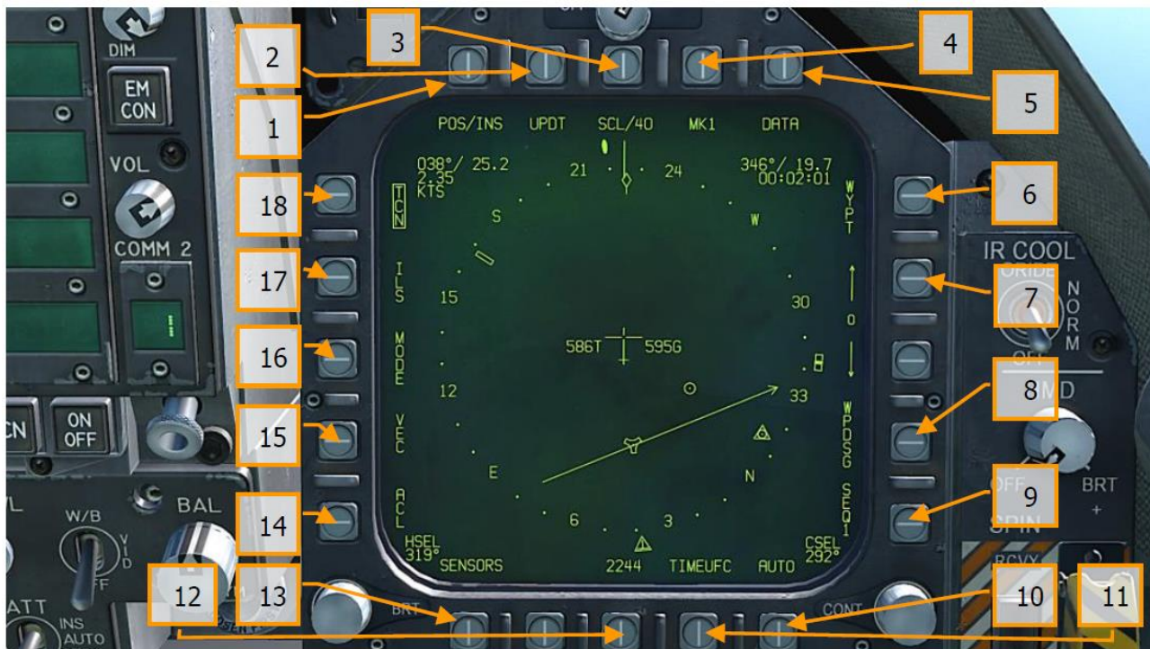
Figure 35. HSI Option Buttons
