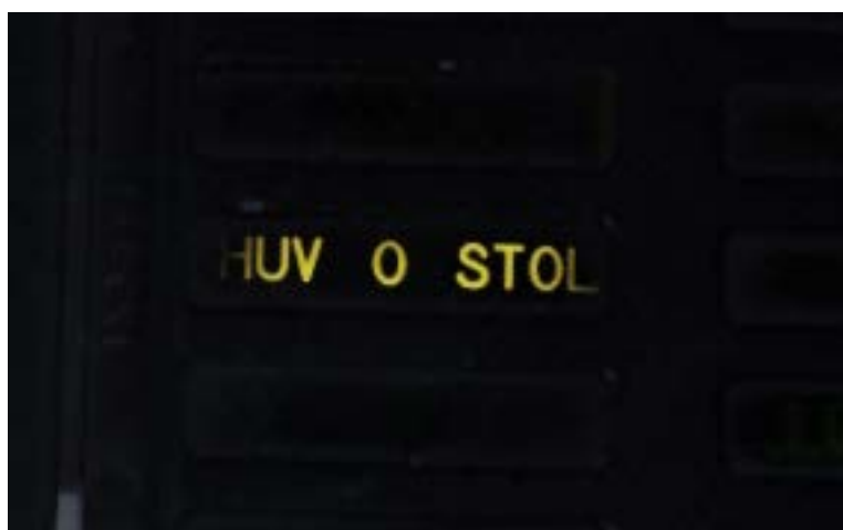
Figure 165 Canopy and ejection seat warning (HUV o STOL)
