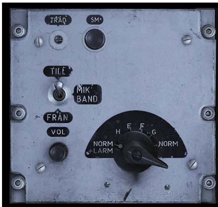
Figure 159 Ground intercom button (TRAD) on the FR24 panel.
