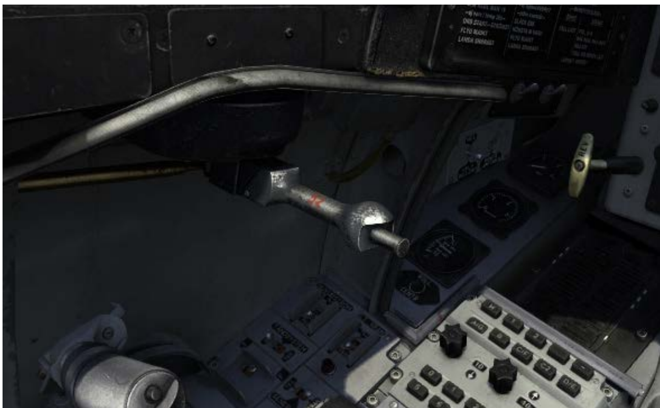
Figure 164 Canopy control lever. In position neutral.
