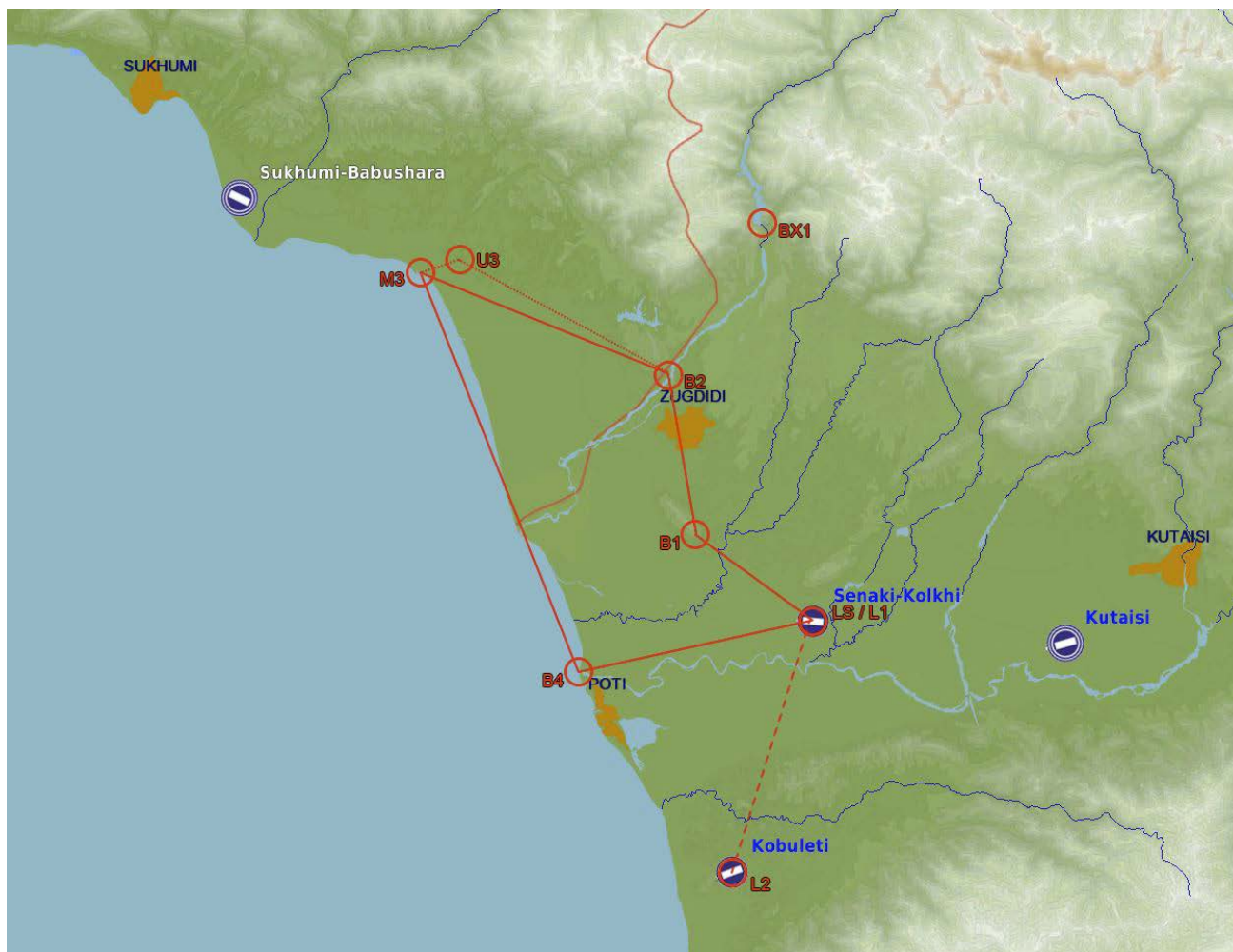
Figure 98 Typical flight plan with 4 waypoints (with a target point M3 assigned). Mark point BX1 added and the optional pop-up point attached to Target point M3 (U3). LS being the starting airfield and the primary landing base (L1) and the secondary landing field (L2)
