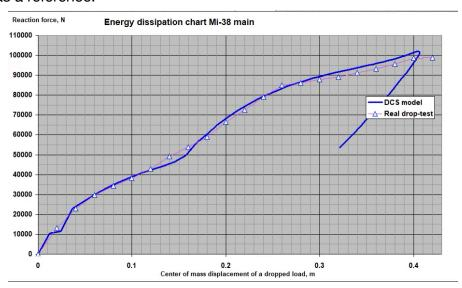
In this test of a two-stage oleo-pneumatic strut, the load mass, initial velocity, and unload factor were known, so a virtual drop-test was conducted under the same conditions.
