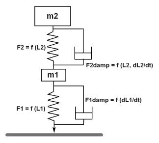
The new model adopts a two-component system, consisting of a strut and a tire in series. This is a classical model, but the main challenge is that it requires numerically solving a second-order nonlinear differential equation. This type of equation involves displacement, velocity, and acceleration (the first and second derivatives).
