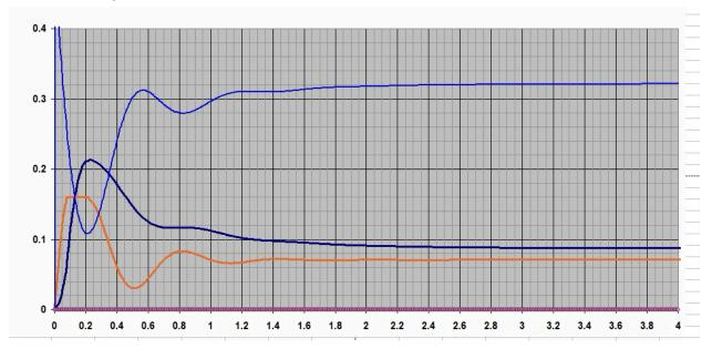
Two things are notable: 1) The strut recoil time is quite long, as mentioned in the report, and the overall process is a superposition of two different transients; 2) The static tire and strut displacements derived from the transient record (tire – 71 mm, strut – 87 mm) do not match the specified on-ground values (47 mm and 63 mm).
