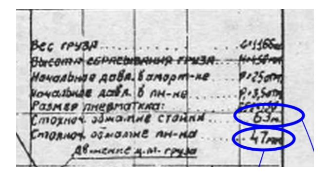
This discrepancy cannot be fully explained, at least not until the full test report becomes available. Nevertheless, it is clear that the transient response for the quasi-linear tire cannot converge to a static displacement of 47 mm given the test data. However, by adjusting the model's dynamic parameters to match the test results, the static parameters can be modified to achieve a static compression closer to 47 mm and 63 mm.
