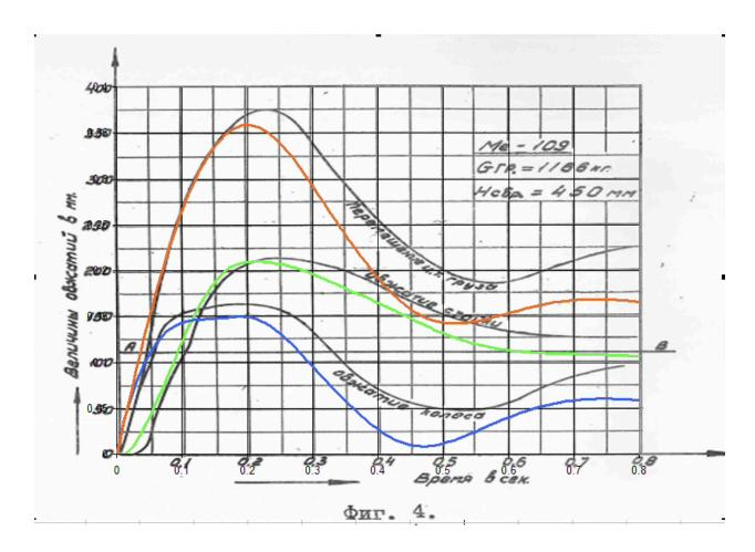
Although we do not have short term plans to develop the 109E, we can extrapolate these results to the 109 G/K series, considering the initial design approaches and the changes implemented for these aircraft. While detailed drop-test or static data is rarely available, we can usually find static, fully compressed, and unloaded displacements for tires and struts, which provides an excellent reference for suspension tuning in our model.
