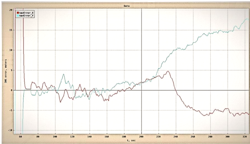
Picture 3. Kalman filter output with INS+GPS signals at its inputs
