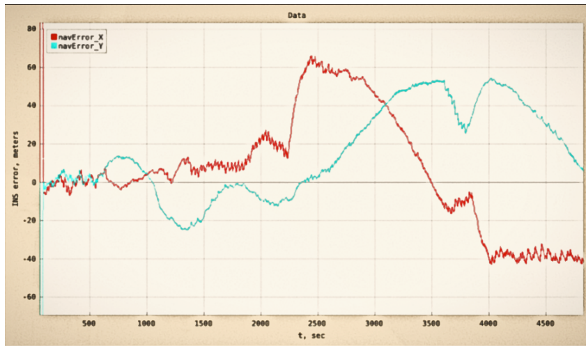
Picture 4. Kalman filter output on a larger time scale
