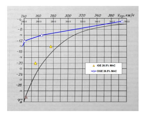
At this point we've come to better understanding of the remark "HA ПОСАДКЕ" (AT LANDING) for that graph Fig. 8.9 from the PA document. It was the common way to provide landing and take-off graphs with the information about gear position and actual flaps/slats deflection. There are some examples when extra IGE graph is also provided as found in MiG-23ML and MiG-21bis manuals.
