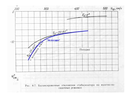
Now it's time to check DCS stability margin curve in landing configuration OGE. It is easy to see that it well duplicates the graph obtained in CFD with only small constant shift.
