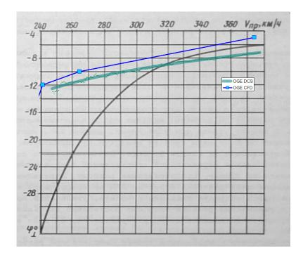
Having accepted the opinion that graph 8.9 is the averaged stabilator deflection, it is possible to export the flight speed and stabilator position from DCS and place these points on the graph 8.9, having previously selected the balancing points by  $n_y = 1 \pm delta$ , where delta is chosen as small as possible so as not to clutter the graph.
