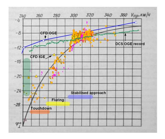
Points of different color on the graph refer to records of different landings. Landings, whenever possible, were carried out with accordance to the recommendations of the Flight Manual and standard landing weight. The green area on the graph refers to the position of the stabilator on the run after touchdown.
