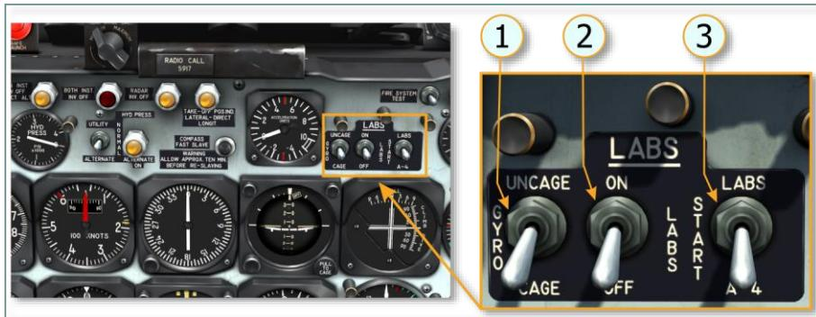
Figure 6.1. LABS Switch Panel
